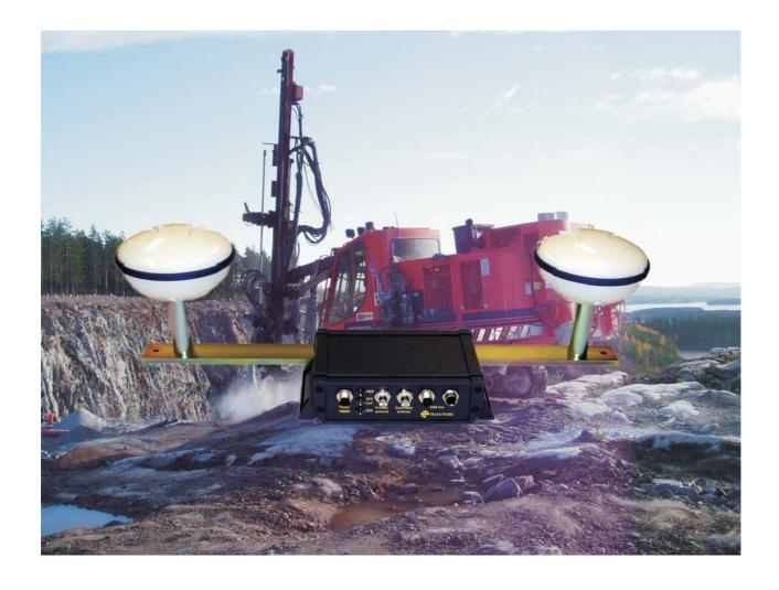
The GPS compass uses GPS satelites to measure the direction of the drill rig with good accuracy. The compass replaces the sight on the CMI bench instrument.
