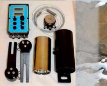
An angle transducer with rollover compensation measures the vertical angle and two boom jointtransducers measure the horizontal angle.
