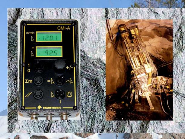
Total instrument system for production drilling rigs with boom mounted feeder.
