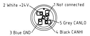
Signal cable connection pin connector Anslutning hankontakt
