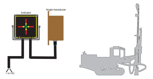
This system is designed to measure the angles on a bench drill rig, drilling vertical holes. It is easy to mount and operate on any type of bench drill rig.
