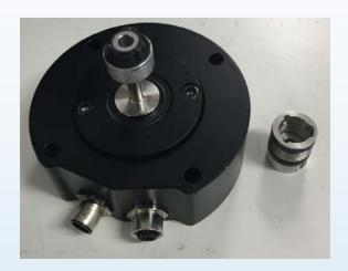
The boom joint transducer measures a non gravity depended angular movement.
